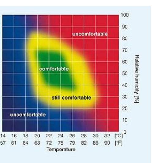
The diagram on left shows the area of temperature and relative humidity witch people would clasify as comfortable and uncomfortable.
