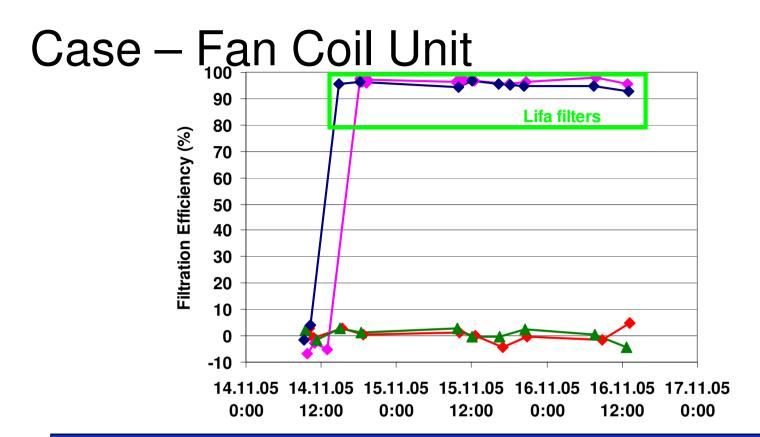
Standard filters in fan coil units do not filter small particles. Above filtration efficiency for 0.3 micro meter particles measured in 4 fan coil units: 2 with standard filters and 2 with Lifa filters.
